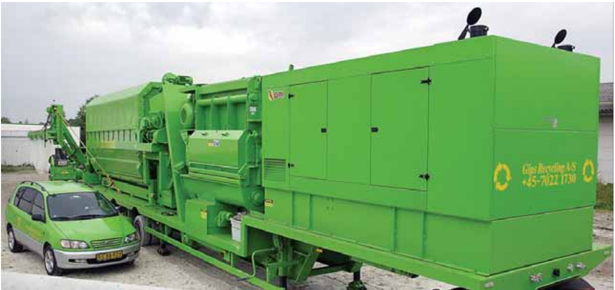
The Cleantech Award winning machine from Gypsum Recycling International cleans and crushes plasterboards for recycling as raw plaster for industrial production.
