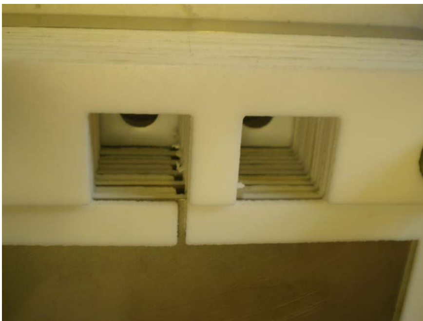
Fig.5.1.8: Hydrogen and oxygen manifold at the top of the stack.
