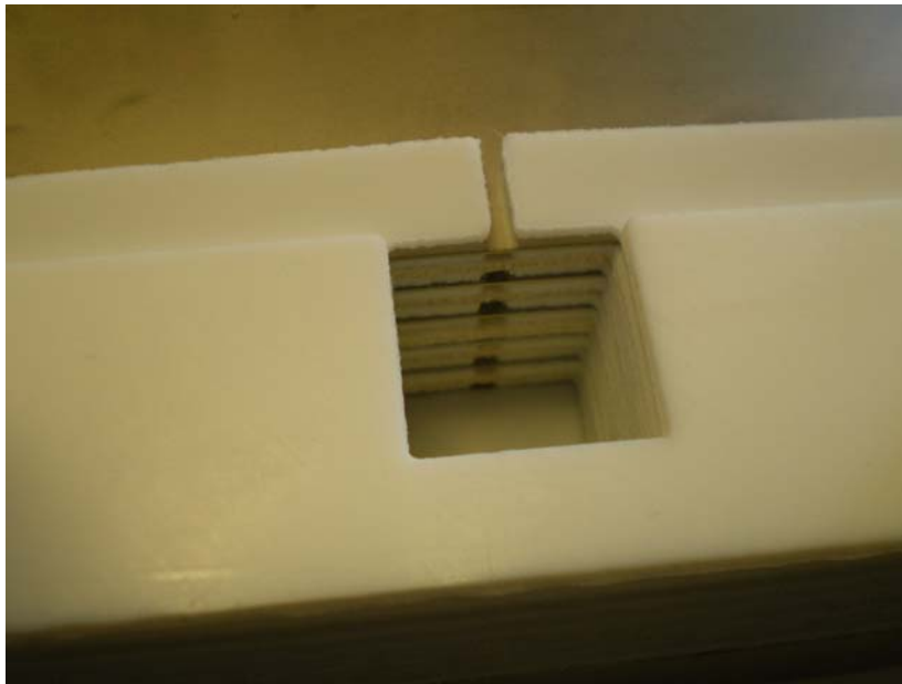
Fig.5.1.9: Electrolyte manifold at the bottom of the stack.
