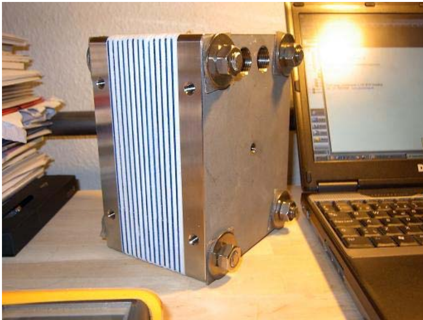
Fig.5.1.7: Test stack with 13 cells
